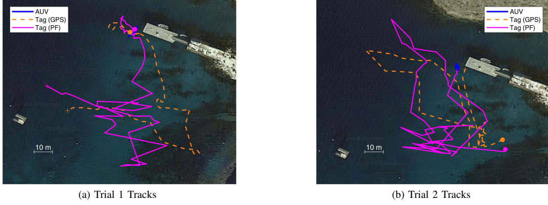
Fig. 6: Overhead view of the tracks in experiments conducted. AUV indicates the location of the AUV; Tag (GPS) indicates the location of the tag logged by the GPS receiver; Tag (PF) indicates the location of the tag estimated by the particle filter. Solid filled circles indicate the start of tracks, and + signs indicate the end of tracks.
