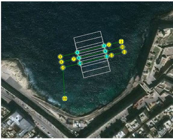
FIGURE 3 Lawnmower trajectory for initial autonomous underwater vehicle search mission [Color figure can be viewed at wileyonlinelibrary.com ]
